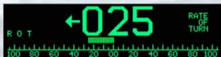
Digital Rate Of Turn and rate of turn indicator. (Degrees per minute).
